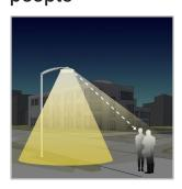
Because of the lower installation height compared to road lighting, visual comfort is an essential aspect of urban lighting. Schréder designs lenses and accessories to minimise any type of glare (distracting, discomforting, disabling glare and blinding glare). Our design offices harness a range of possibilities to find the best solutions for each project and ensure that we provide a gentle light that delivers the best night-time experience.
